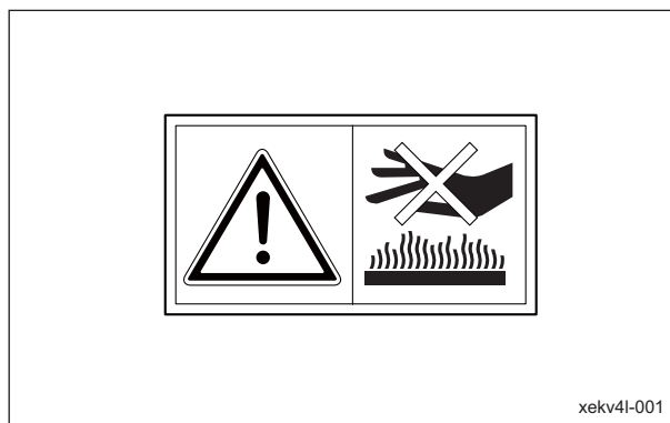
Caution for High Temperatures Decal_001
