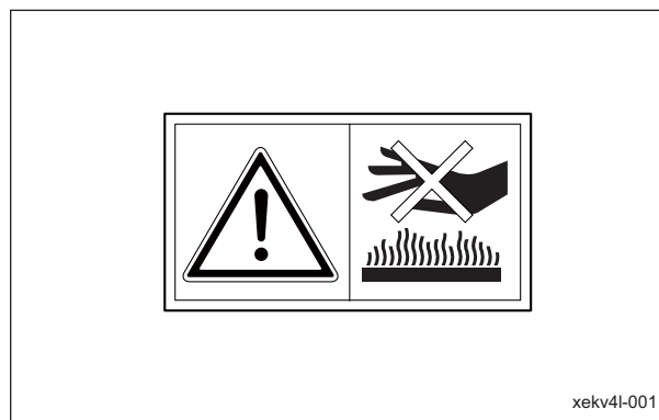
Caution for High Temperatures Decal_001
