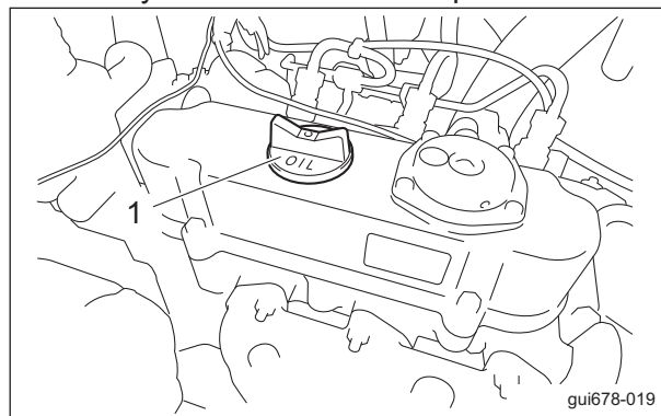
Replacement of Engine Oil_002
