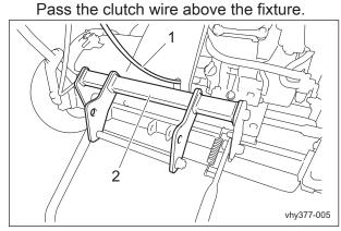
Installation of Greens Mower Fixture\_005
