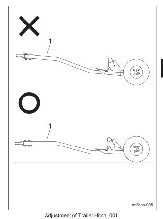
The hitch can be adjusted to one of three heights.
