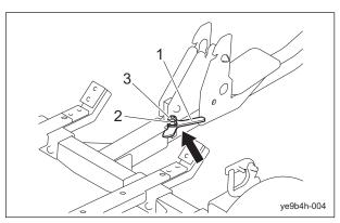
Adjustment of Axle Lock Lever\_001
