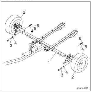
Adjustment of Tread Width (Mower Drums)\_001
