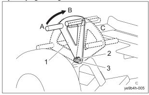
Adjustment of Mower Tire Lock Lever\_001
