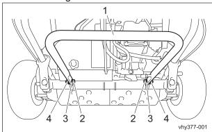
Installation of Greens Mower Fixture\_001
