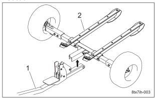
Connection between Towing Section and Axle Section\_001
