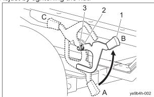
Adjustment of Drum Shaft Lock Lever\_001
