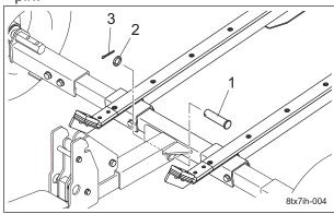
Connection between Towing Section and Axle Section\_002
