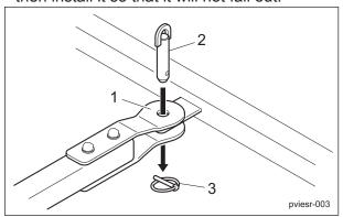
Connection Method of Mower Trailer\_003
